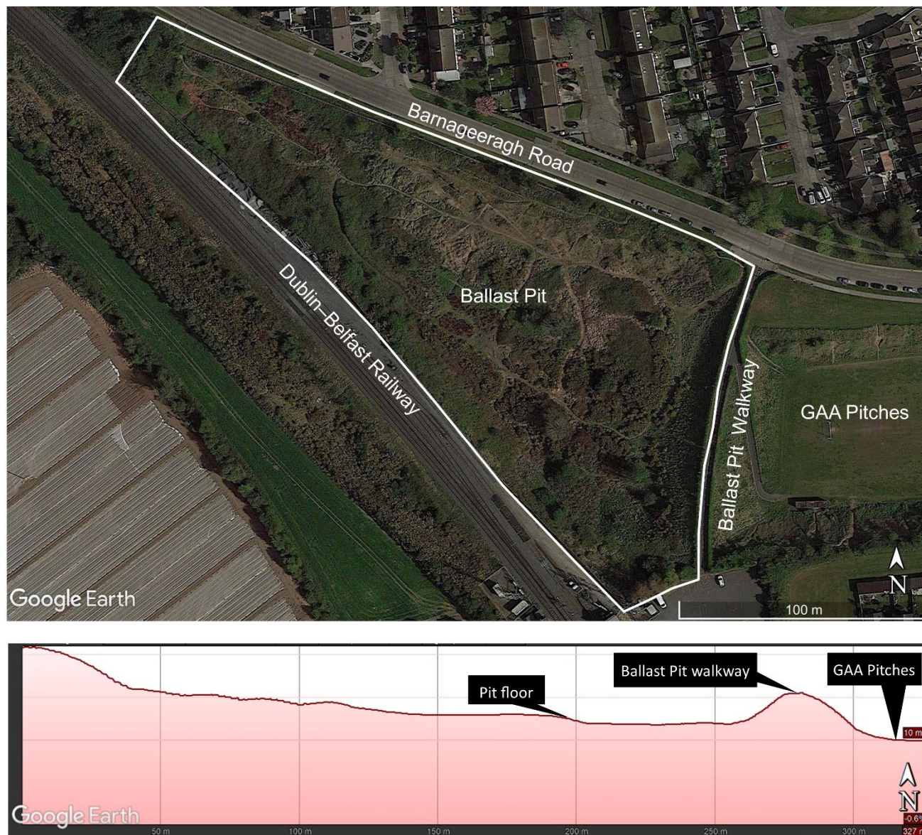
Figure 2. Aerial view of the Ballast Pit (above); longitudinal section/profile looking north (below).
